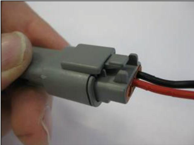
6. Plug the other end of the remote engage adapter cable into the port replicator (pin 10 and pin 11) on the EZ-Pilot cable that is connected to Port B on the CFX-750 display:
