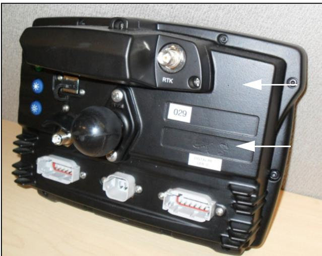
2. Attach the RAM mount to the ball on the diamond-shaped mounting plate:
