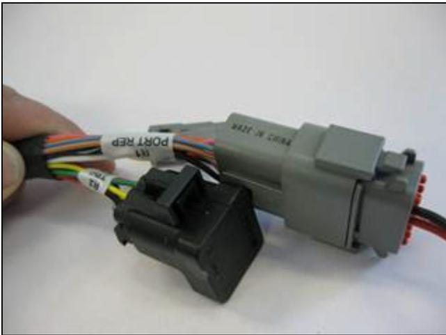
**Note** – If you are using a sonalert, you must remove engage pin 10 and move it to pin 8 so that the remote engage functions run between pin 8 and pin 11 and the sonalert functions between pin 2 and pin 10.
