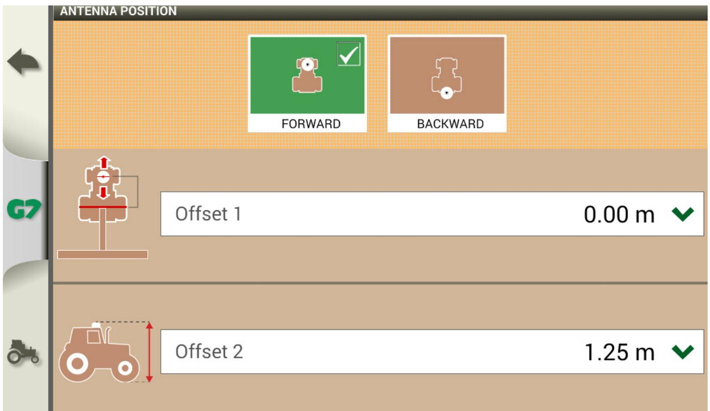
Figure 2.3.1.c - Antenna position settings
