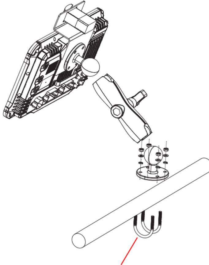
Secured to the tubular section of the vehicle with U-bolts.
