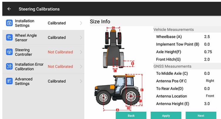
**Wheelbase of front and rear wheels (A):** Measure the distance between front wheel rotation axis and rear wheel rotation axis. Note that the tape measure needs to be parallel to the ground.
