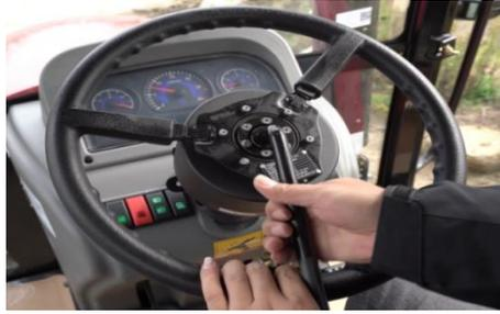
f) Screw the T bracket to the T mount kit tightly with M10 nuts (2 pcs);
