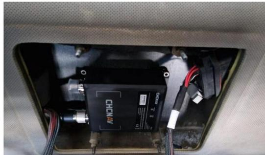
2. Find the 40-pin Deutsch connector on the tractor rear side(Different location for different vehicles)
