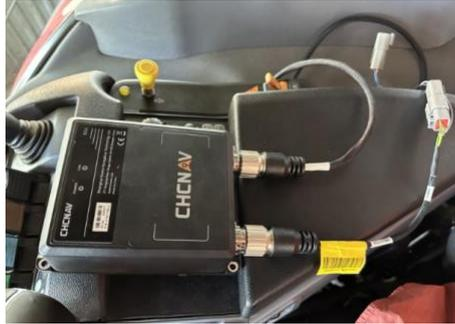
5. Connect to power with NX510 main cable in the tractor cab or tractor battery depending on users.
