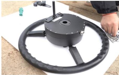
c) Fix the T mount kit to the shaft with M8\*60 hexagon screws (2 pcs);
