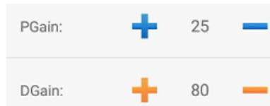
**PGain:** Motor Adjustment speed ratio. The smaller the value, the slower the adjustment.
