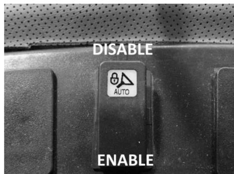
6. The vehicle is equipped with a guidance engage button. Press the button to engage/disengage the auto steer system. The operator can either engage the autosteer with the button switch on the console or with the display.
