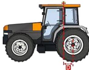
**Antenna Location:** The relative position between the antenna center(the position of the antenna center should be referred to the blue indicator) and the rear axis. Select **Front** if the antenna is in front of the rear axis, select **Rear** if the antenna is behind the rear axis.
