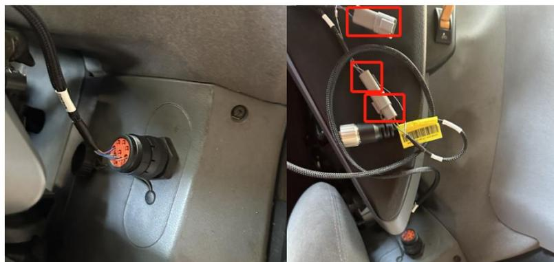
4. Connect to CHC PLC controller COM2 with another end of CANBUS cable1 (4103020173), also connect to PLC controller COM1 with another CANBUS cable2 (4103020172) connecting to motor interface of NX510 main cable for supplying power and data communication.
