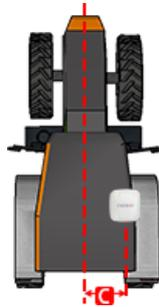
**Antenna position of C:** Fill in according to the receiver position.
