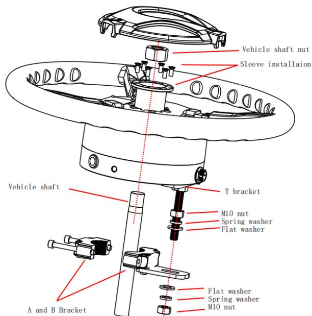
a) If the sleeve can fit the spline, please remove the protective cover of the steering wheel, place the sleeve in it, and fix the sleeve with M5\*11 phillips screws (6 pcs);
