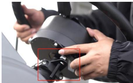
e) Hold the steering wheel and tighten the spline screws with tools;
