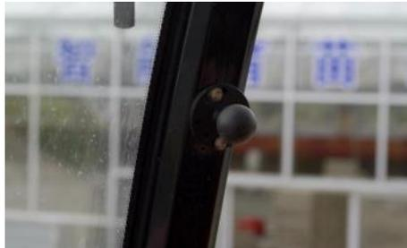
c) After complete the installation, it is available to adjust the tablet to a suitable position;
