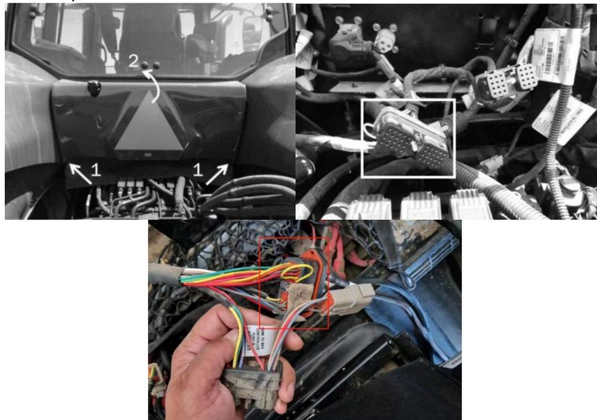
3. Open the hood by pulling on the latch and lifting on the handle located at the front of the hood. Route the black 2-pin Deutsch enable solenoid connector on the Interface. Cable under the right side of the cab up to the factory steering valve where the enable solenoid is located.
