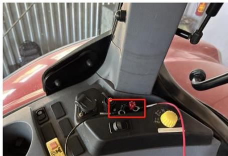
6. Install NX510 PA-3, camera and tablet, etc on the top of tractor as the regular procedure, the place is better to close to rear axle, also PLC controller can be installed at the any place in the cab without leveling or some special notifications.
