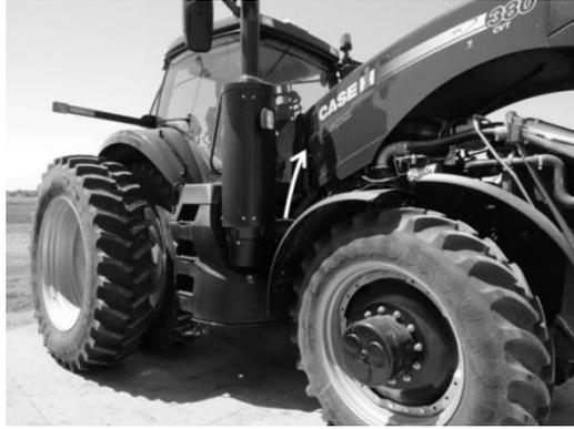
4. From the right side of the vehicle, reach over to the left side of the factory steering valve and unplug the factory 2-pin Deutsch enable connector. Plug the 2-pin Deutsch connector in place of the factory connector.
