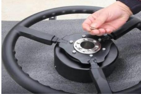
b) Install T bracket or standard bracket on the motor with M5\*16 hexagon screws (2 pcs);
