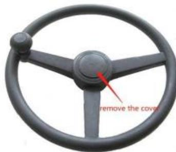
b) Stabilize the steering wheel, use the sleeve tool to loosen the original vehicle spline screws, and remove the original vehicle spline screws;
