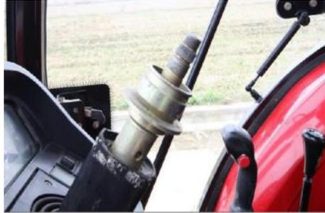
d) Before install the sleeve into the steering wheel, please try it on the spline to check whether the size fits.
