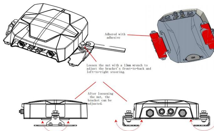
a) The receiver needs to be installed on the central axis of the vehicle roof as possible, and the installation direction should be parallel to the vehicle as possible;
